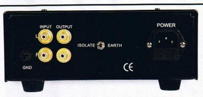
ABOVE: Gold-plated RCA sockets are used throughout. The P10 features an earth lift switch to obviate hum loops should they occur, while the T10 offers a choice of 36 or 144ohm loading
